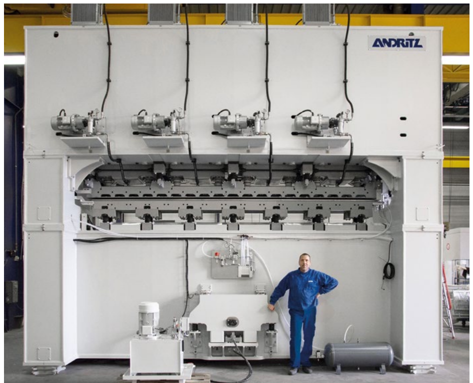
Rib structuring SDB in 4.4 m working width
