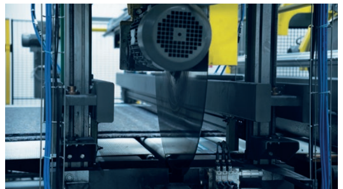
Edge trim recycling unit in operation
